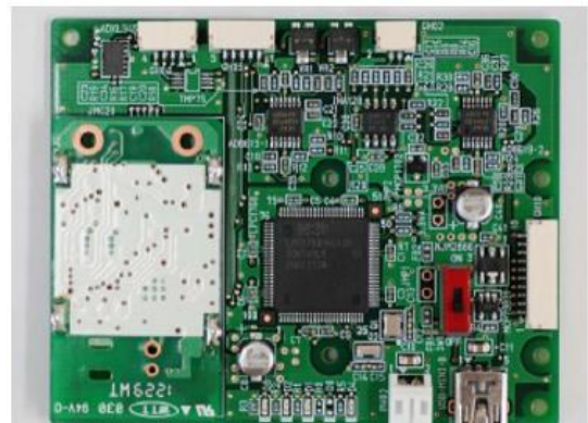
Fig. 3. Photo of the vital sensor node on the PCB.
